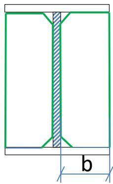
$$\text{Para ASTM A36} \quad \frac{b}{t} < 16$$
